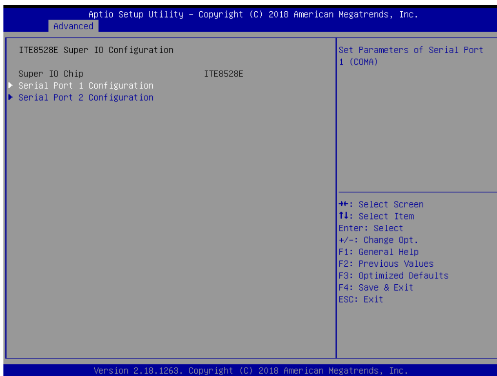
Figure 3.5 Super I/O configuration setup screen
