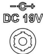
Figure 2.8 DC input connector
