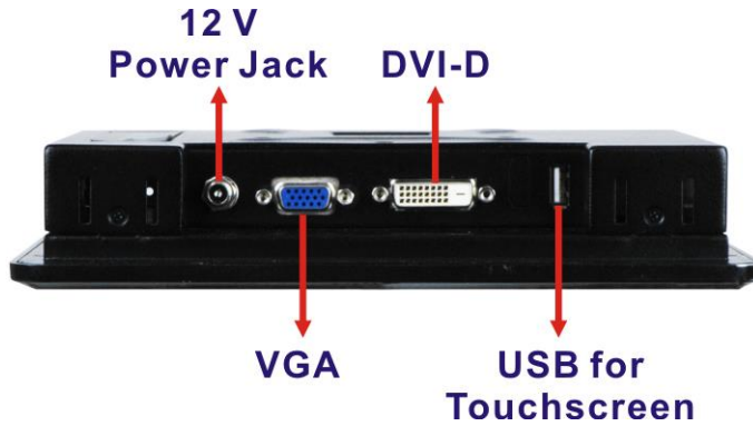
Figure 1-5: Bottom Panel Connectors (DM-F08A)
