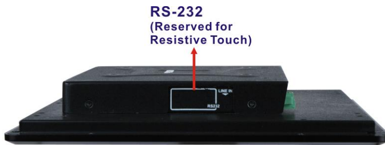
Figure 1-8: Side Panel Connector (DM-F12A/15A/17A/19A)
