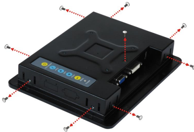
Figure 3-9: Rear Panel Retention Screw Removal (DM-F08A)
