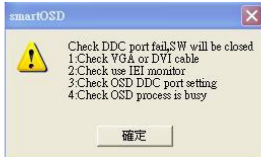
Figure C-18: DDC Port Failure
