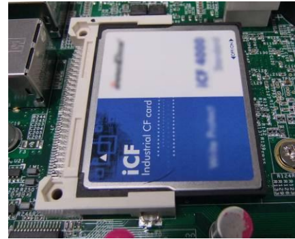
Fig. 6-2 Push Compact Flash Card into the CF interface
