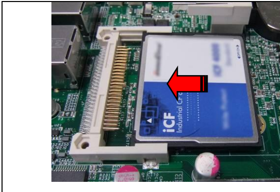
Fig. 6-1 Insert Compact Flash Card
