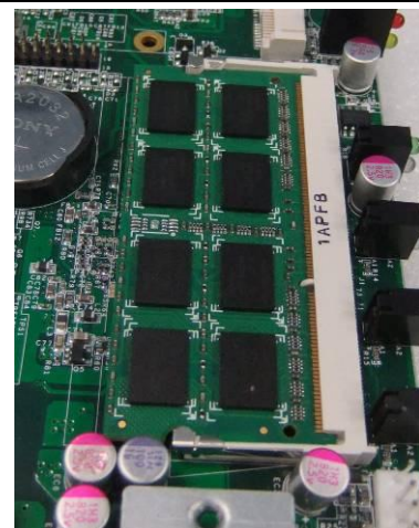
Fig. 7-2 Press down the memory module into socket
