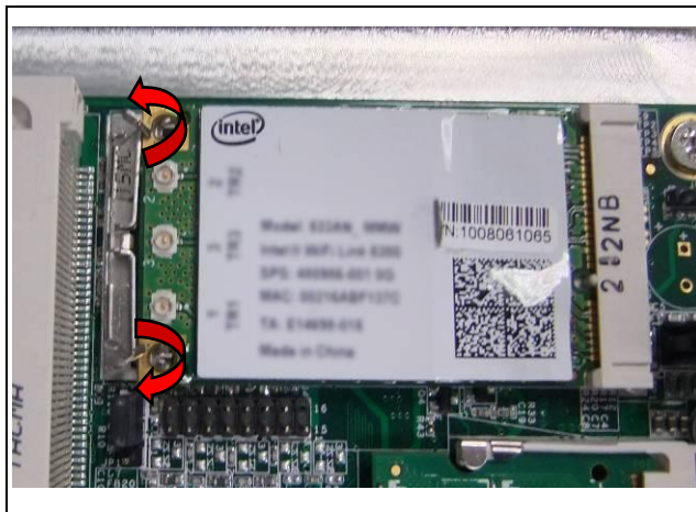
Fig. 9-3 Release two clips to remove module
