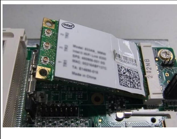
Fig. 9-1 Insert Mini PCI-e module (Supports USB signal only)
