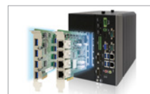
Support add-on GPU graphic cards and LAN/ PoE/USB3.0 I/O cards
