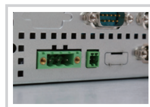
DC/AC Power Input, Support AT/ATX Mode
